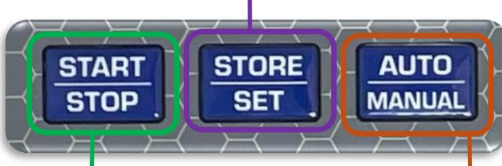
A short press of START/STOP switches the unit between standby and active. The pump icon animates when power is being supplied to the pump
